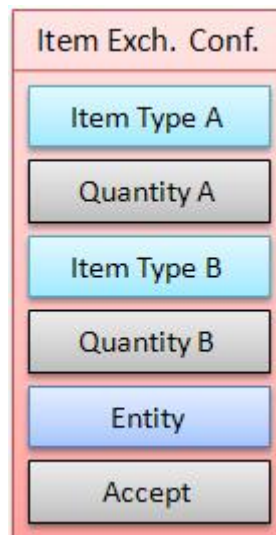
Figure 28 : Message Item Exchange Confirmation structure
