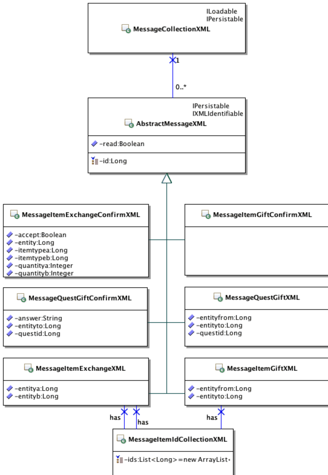
Figure 53 : UML – Messages XML classes
