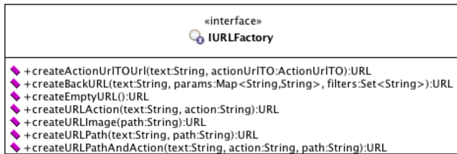
Figure 81 : UML – IURLFactory interface
